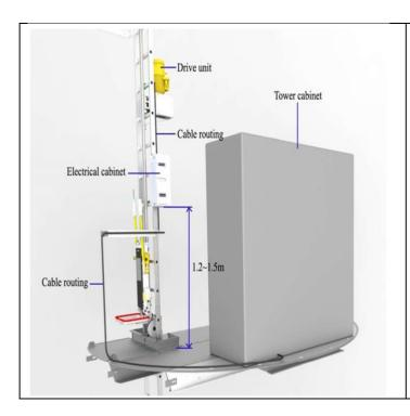
Power supply type is single phase 240V, 50Hz. The distance from the Climbing system to power supply is 2 meters.
