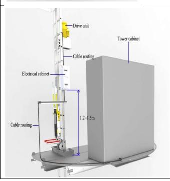
Power supply type is single phase 240V, 50Hz. The distance from the Climbing system to power supply is 2 meters.
