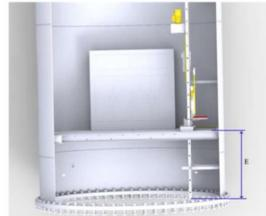
The top anchor point of the existing cable type fall protection system on the ladder is removable.
